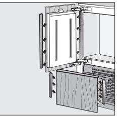
To mount the cover strips on both sides of the upper and lower doors, click them into place from bottom to top, into the gap between the appliance door and the custom door.
